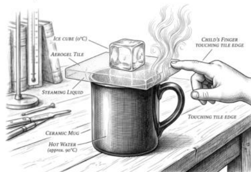
PLATE 24. THERMAL INSULATION DEMONSTRATION OF AEROGEL.
